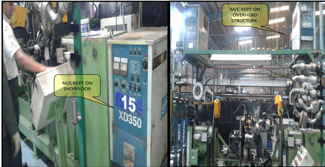
Figure 4.35 Overhead platform in Scorpio muffler assembly line
